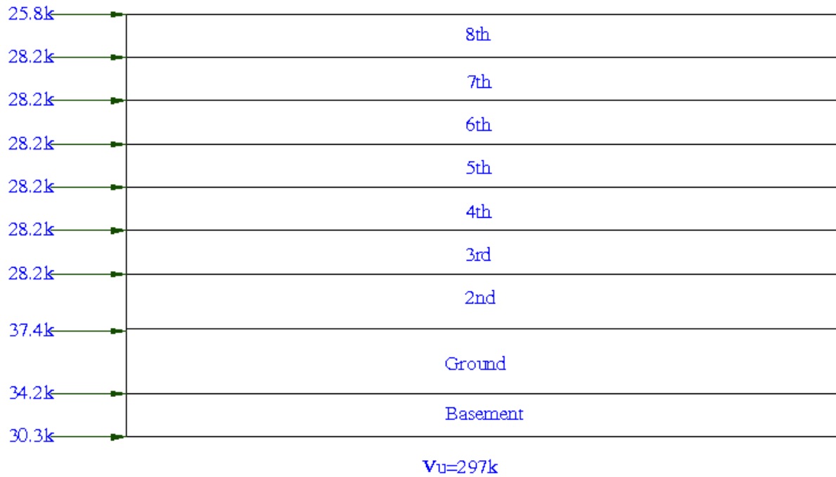
Figure 7: Seismic Loads on East-West face
